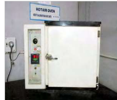
Hot Air Oven MSFRT-02 | Range: 0°C to 1000°C
