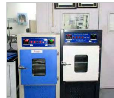
Conditioning Chamber CC-01, CC-02 Range CC-01: 20°C-40°C, 54-99% RH Range CC-02: 20°C - 40°C, 40-70% RH
