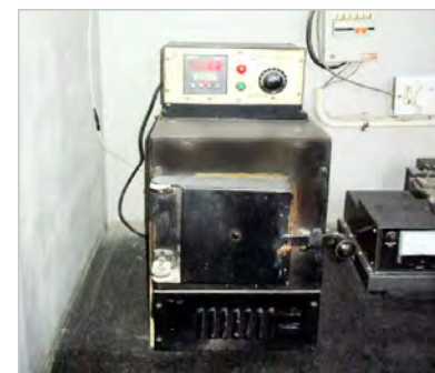
Muffle Furnace MSFRT-3 Range: 0°C to 1000°C
