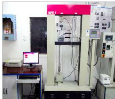
Universal Testing Machine MSFRT-1 Tensile Load Capacity-5000 kg Flexural Load Capacity-225 kg
