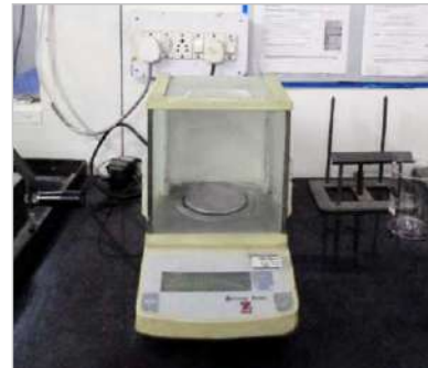
Weighing Scale MSFRT-02 | Range: 0g to 200g
