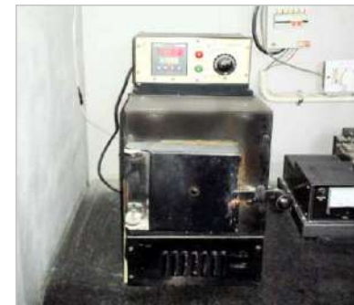
Muqe Furnace MSFRT-3 Range: 0°C to 1000°C
